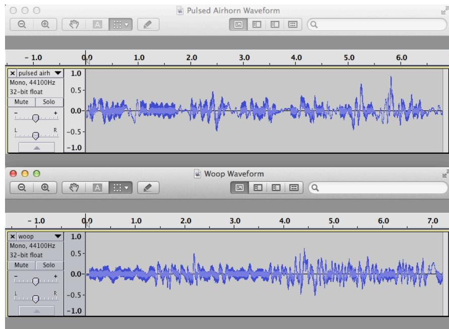
**Figure 3-4:** “Pulsed Airhorn” (top) and “Woop” (bottom) waveforms. The x axis represents time in seconds and the y axis represents digital volume. The digital volume ranges from -1 to 1 beyond which the signal will be distorted due to clipping.
