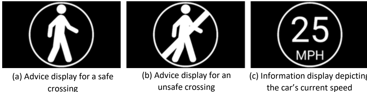
Figure 2: Proposed displays to aid pedestrians in making road crossing decisions in the presence of self-driving cars.
