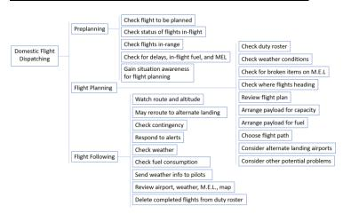
Figure 3. Flow chart for domestic flight dispatching.
