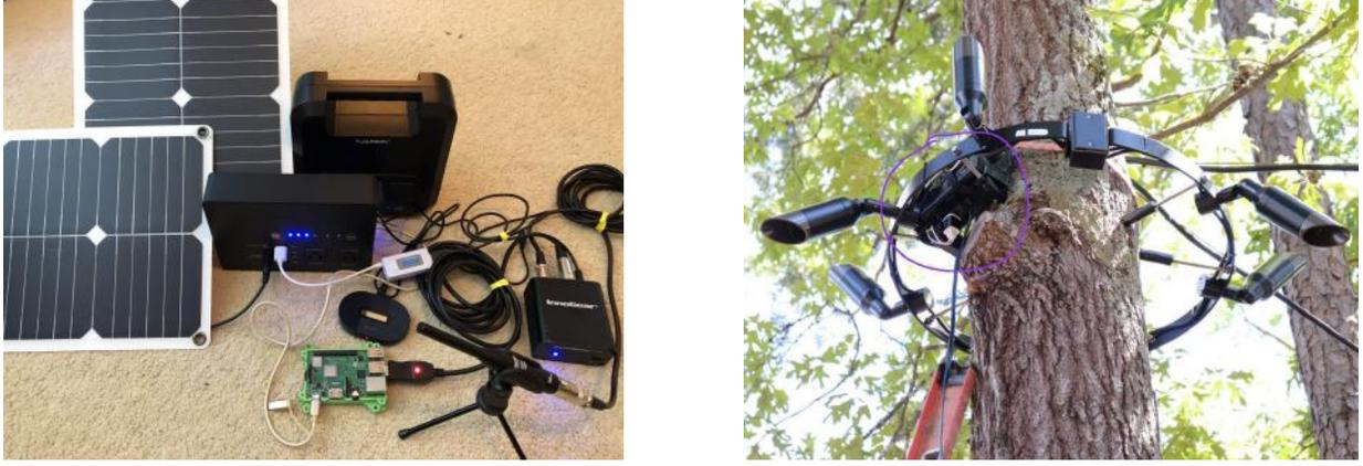
**Fig. 2** (a) The acoustic signal detection system that includes a microphone, a Raspberry pi with timer, and optionally solar panels, (b) Appearance of the system when installed inside a waterproof box powered by conventional AC.
