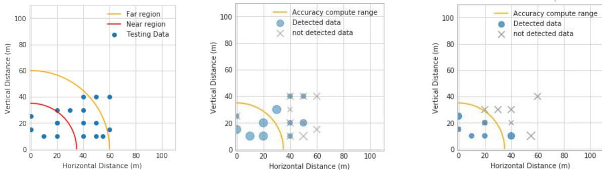
**Fig. 8 Dan River Work Farm static test plan and results (a) Static test coordinate points (b) Phantom 4 Pro static testing results and (c) Mavic Pro static testing results. Size of markers represent the number of predictions.**
