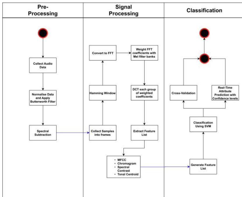
Fig. 1 Flow chart for acoustic detection and classification.
