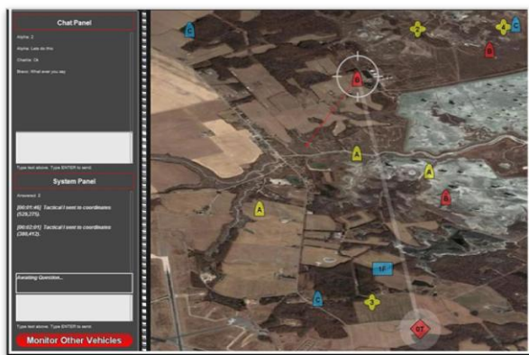
Figure 3: Main display of the ground control interface.
